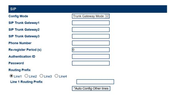
The device accepts calls from up to 3 IP addresses (SIP Trunk Gateway1, SIP Trunk Gateway2, SIP Trunk Gateway3) specified and then dial out the call via an Idle channel that is used the least (in terms of the number of calls dialed). The last part of the SIP Trunk Gateway IP addresses can be specified as "X" or "x" to represent that the whole segment IP addresses (0 - 255). Calls originated from the IP segment are accepted.
