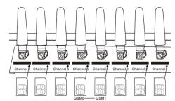
For GoIP-16, the SIM card insertion orientation is shown in the figure below. The cut corner is pointing downward with the metal contacts facing the front of the GoIP.
