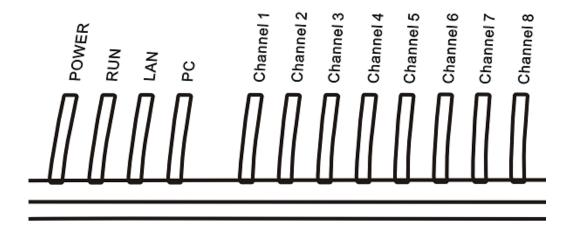
LED indicators (shown above for GoIP-8) are used to show the current status of the device. They are often used to determine if the device is working normally or not.
